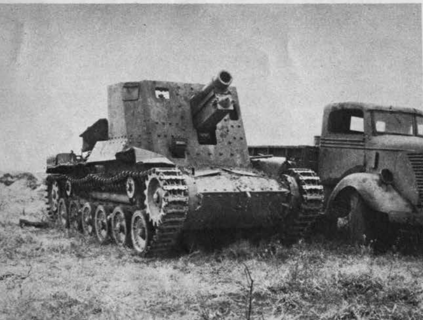
Familiar Model 97 chassis also carries 150-mm. howitzer, recently recovered on Luzon. Mount on right of vehicle may be for MG.
